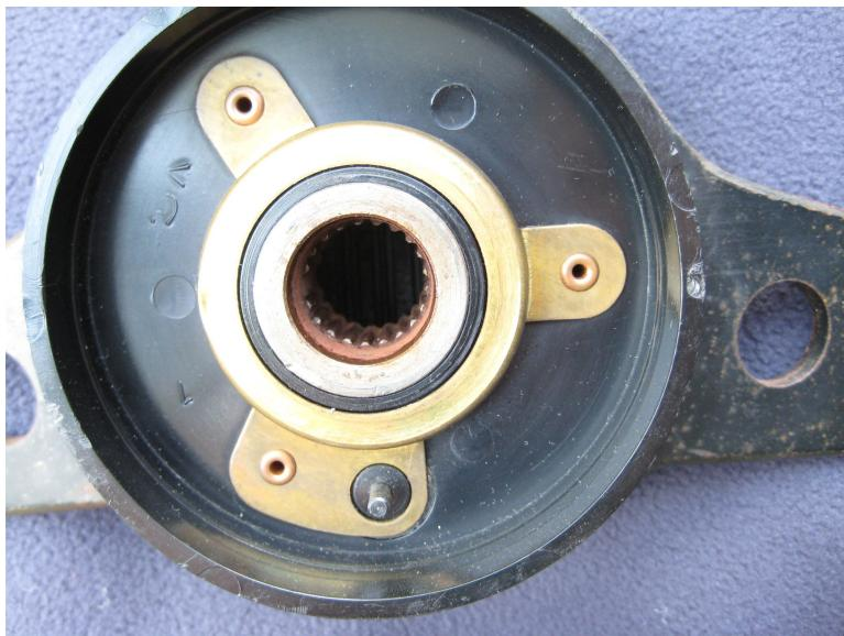
As you can see, the wheel has 21 notches which match up with another 21 notches on the top of the steering column:
