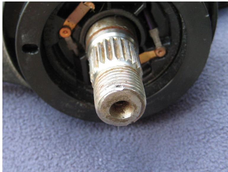
The steering column then attaches to the car with a 17 notch connector:
