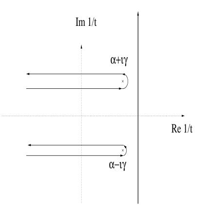
Rightmost singularity(ies) of NS solution  $\hat{v}(k,t)$  in the 1/t plane determines optimal  $\alpha$ .  $\gamma$  gives dominant oscillation frequency.
